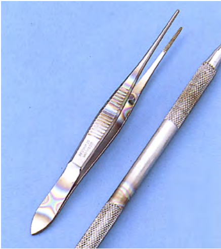
Contact corrosion due to preparation on a brass rack
