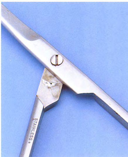
Fretting corrosion due to insufficient treatment with oil
